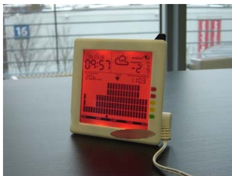
Figure 7: Energy traffic light device showing the existing and future energy prices
