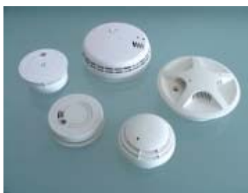
Figure 5: Typical household smoke detectors with integrated nP2M-module
